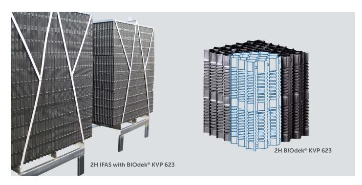
IFAS (Integrated Fixed Film Activated Sludge) combines the advantages of fixed film technology i. e. submerged fixed beds (SAF) and conventional activated sludge (CAS). By adding high surface media to an activated sludge basin additional biomass will grow on the media increasing the operative sludge age. Thus, IFAS offers a possible performance increase up to 40% without new aeration tanks.
